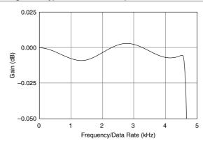
Figure 2. Typical Passband Response for the NI 9236
